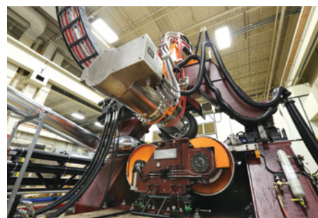
The Flat-Trac LTRe features an electric spindle torque drive that delivers the power density and ultra-high performance bandwidth required to apply driving and braking torque at full roadway speeds, under physical loads up to 30,000 N in all three force directions.
