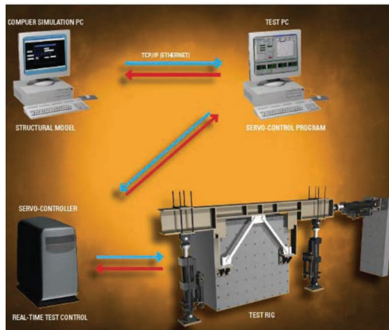
Quasi-static Hybrid Simulation System Diagram
